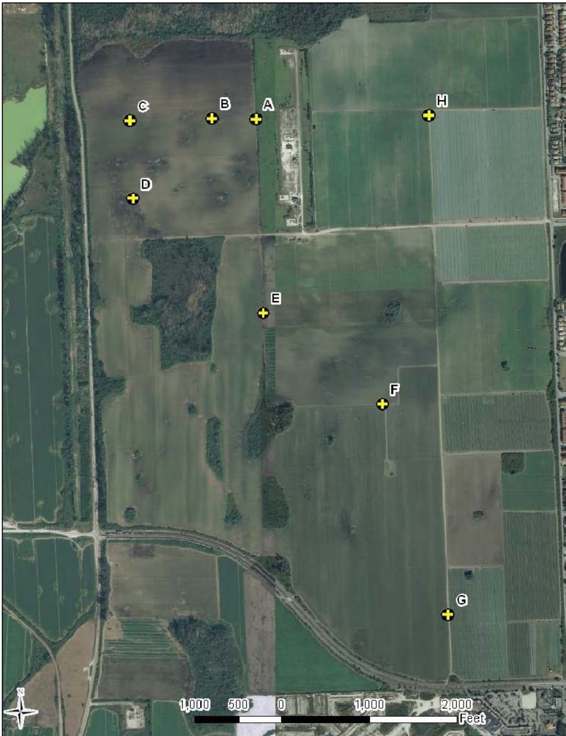
AERIAL VIEW OF SITE SHOWING LOCATION OF GROUNDWATER PIEZOMETERS INSTALLED AND MONITORED BY CRB
